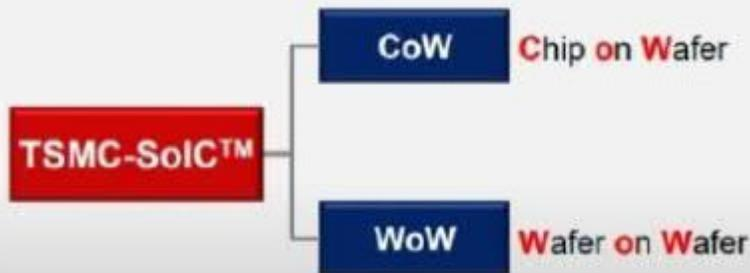
SoIC: System on Integrated Chips
